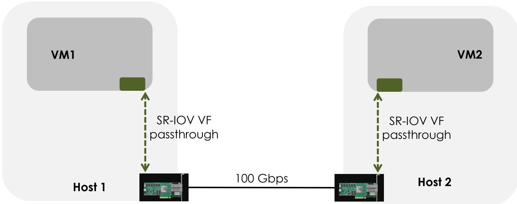
VMs receive a SR-IOV VF in passthrough, i.e., a hardware slice of the NIC.
